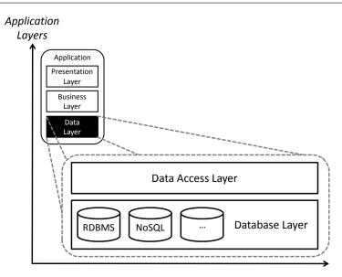
Fig. 3 Subdivision of the Data Layer into Data Access Layer and Database Layer
