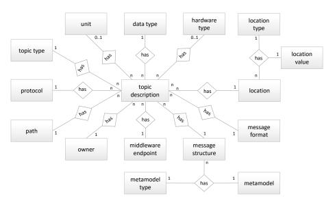
Figure 3. Data model associated with the TDLIoT
