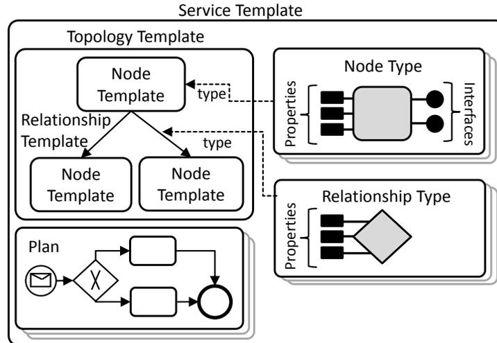
Fig. 1. Overview of TOSCA Building Blocks (adapted from [1])
