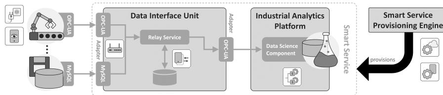
**Fig. 6.** The final example system after applying the REMOTE PROCESSING and LOCAL PROCESSING patterns.
